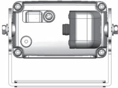
**2** Assemble the camera loosely to the bracket.
