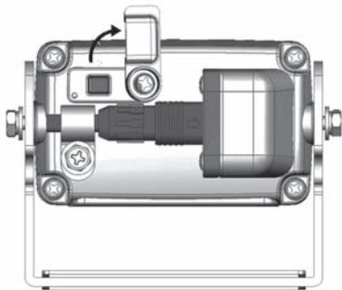
**Changing the Camera Image:** If you need to reverse the camera image, you can do so by loosening the screw on the Image Reversal Switch cover located on the back of the camera. With the screw loose, simply rotate the cover out of the way and press the switch.
