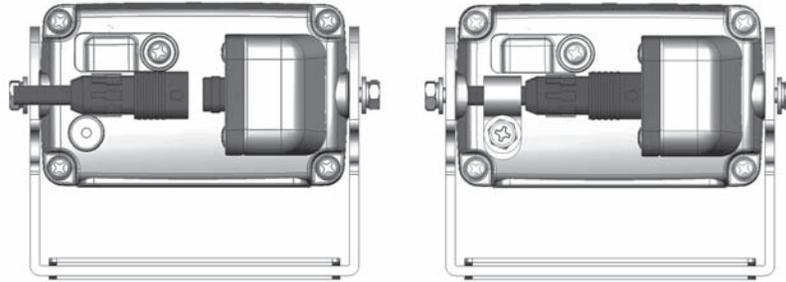
**3** Connect the cable by aligning the alignment marks on the connectors and push together until locked. Secure cable with the "P" clamp provided.
